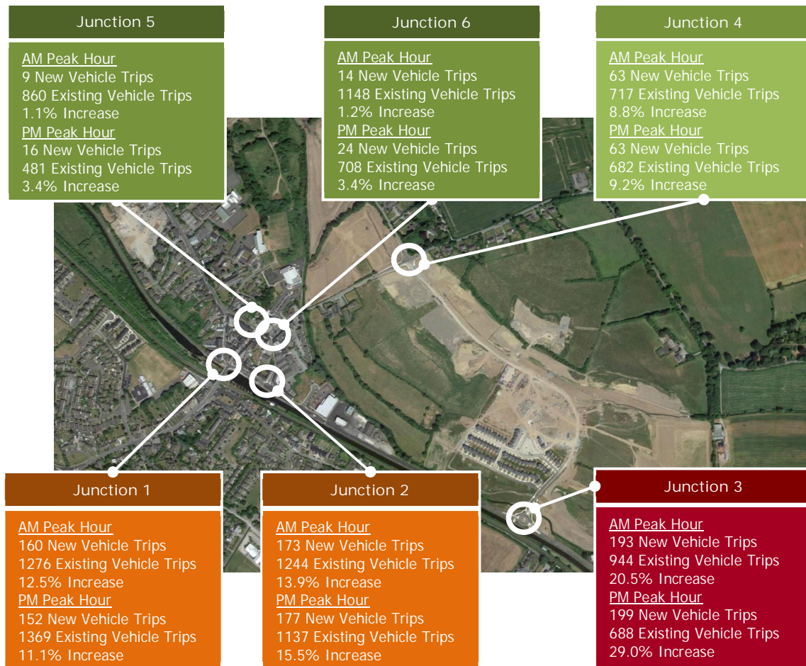
Figure 5.3: Increase in Vehicle Trips Generated Through Key Local Junctions (2036 Future Design Year)
