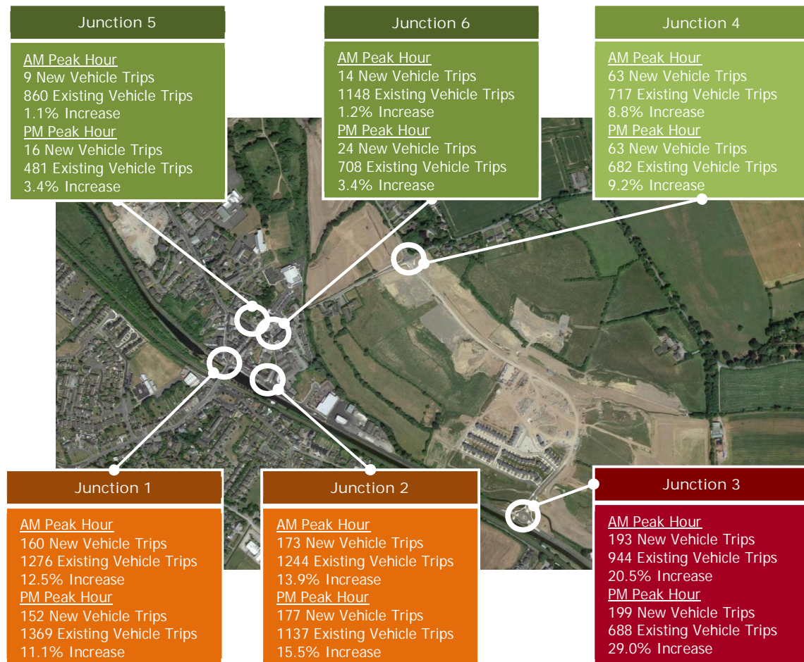
Figure 7.1: Increase in Vehicle Trips Generated Through Key Local Junctions (2036 Future Design Year)
